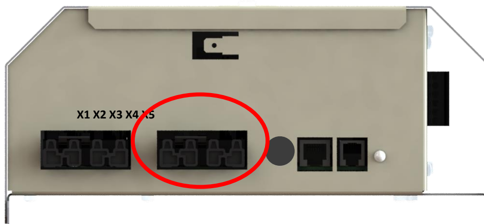
Figure 17: Socket X2 Power Supply Laboratory Fume Hood Light – Output Laboratory Fume Hood Light
