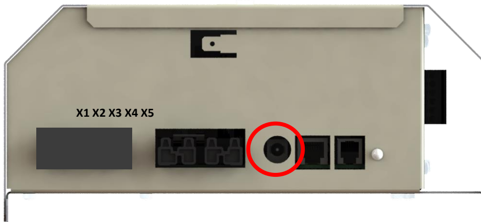
Illustration 19: Socket X3 power supply with external supply 24 V DC
